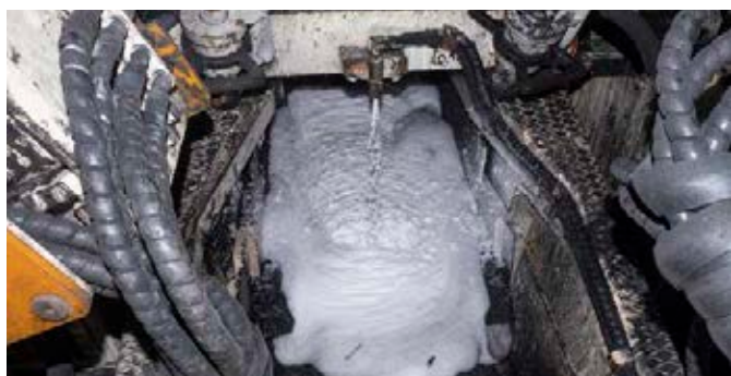
Picture 1: The dust suppression system uses biodegradable foam is applied to coal as it moves through mining machinery during the development phase of mining. The system binds to coal and significant reduces coal dust exposure. This technology won the Queensland Health and Safety Award for Innovation in 2018
